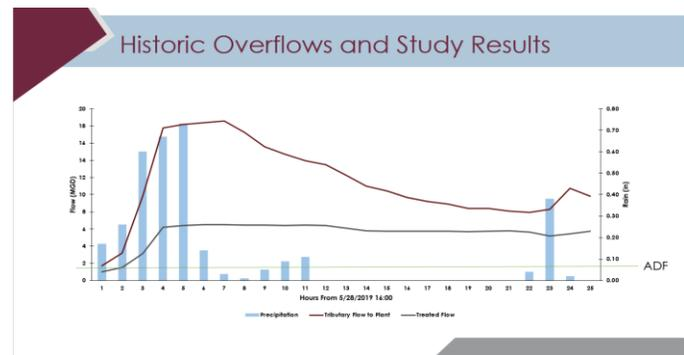
Data illustrated in this graph is the result of a flow study with data collected during a May 2020 storm event and highlights the WPCP average daily flow (static green line) versus the tributary flow to plant in millions of gallons per day (red line)
